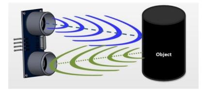
Figure 6: Ultrasonic sensor
