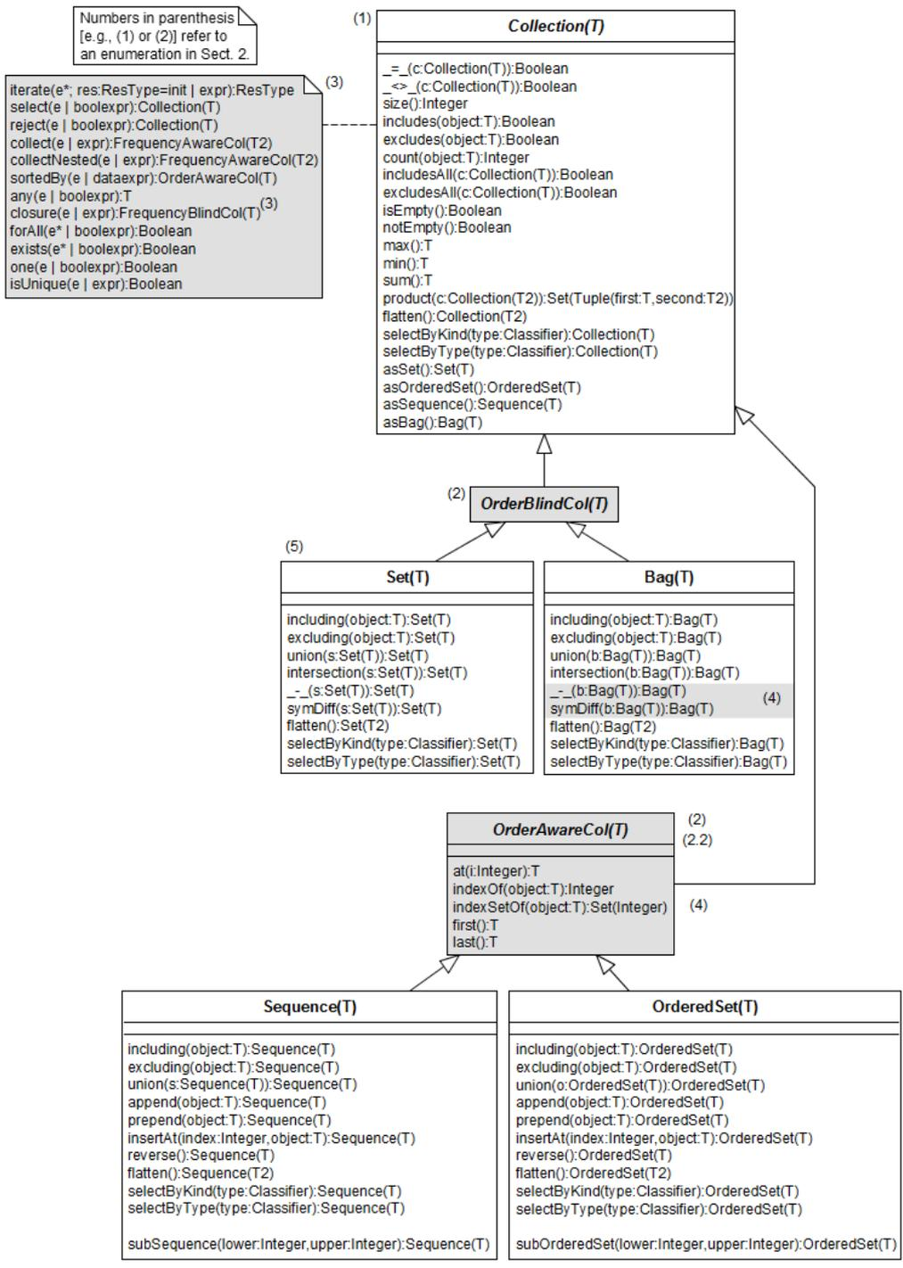
Figure 4: Refactoring Collection Kinds and Operations for OCL.
