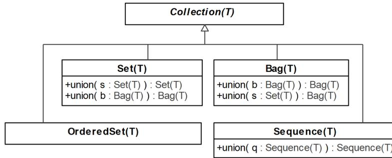
**Figure 1:** Operation `union()` in current OCL Collections specification.
