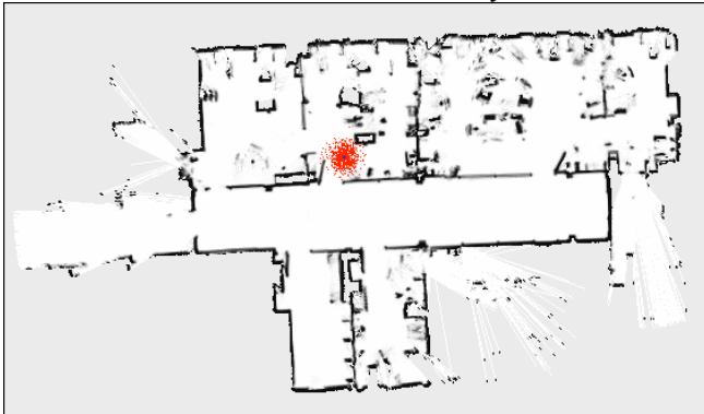
Figure 5. Example of a 2D map created using LiDAR data. The red blob represents the region where a robot is currently located in the map (ref. agv-iit-kgp.github.io , IIT Kharagpur, in [Madan and Gauthey, 2017]).
