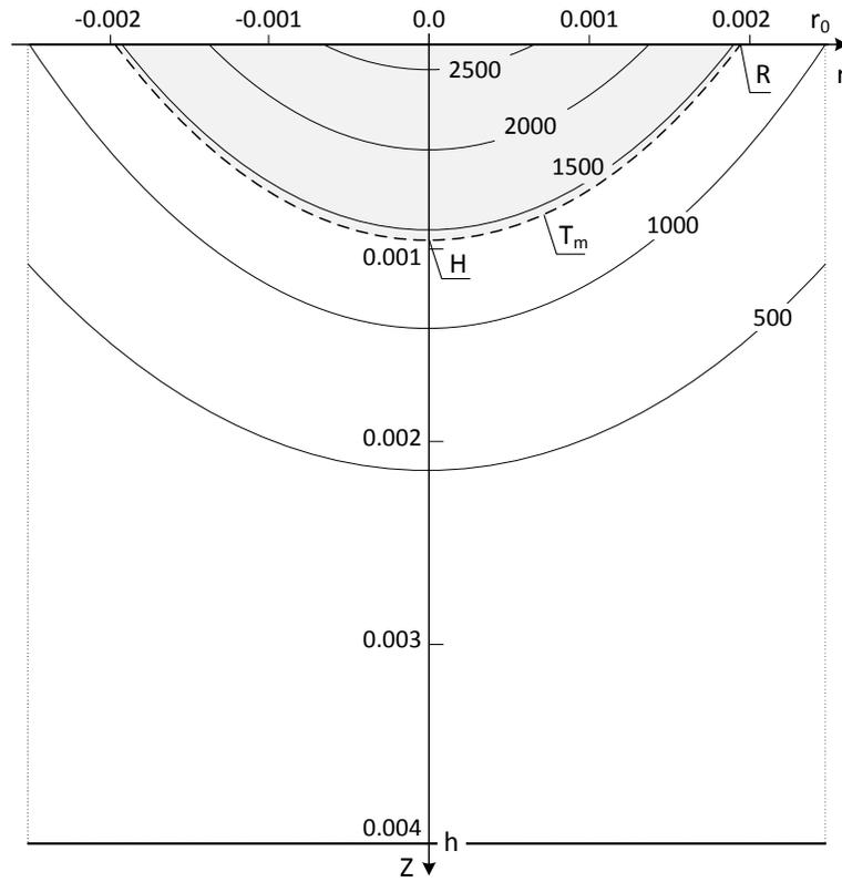
**Fig. 3.** The diagram of temperature distribution across the processed sample height. The dark area limited by dashed isotherm  $T_m$  corresponds to the molten pool with a depth  $H$  and radius  $R$  on the sample surface
