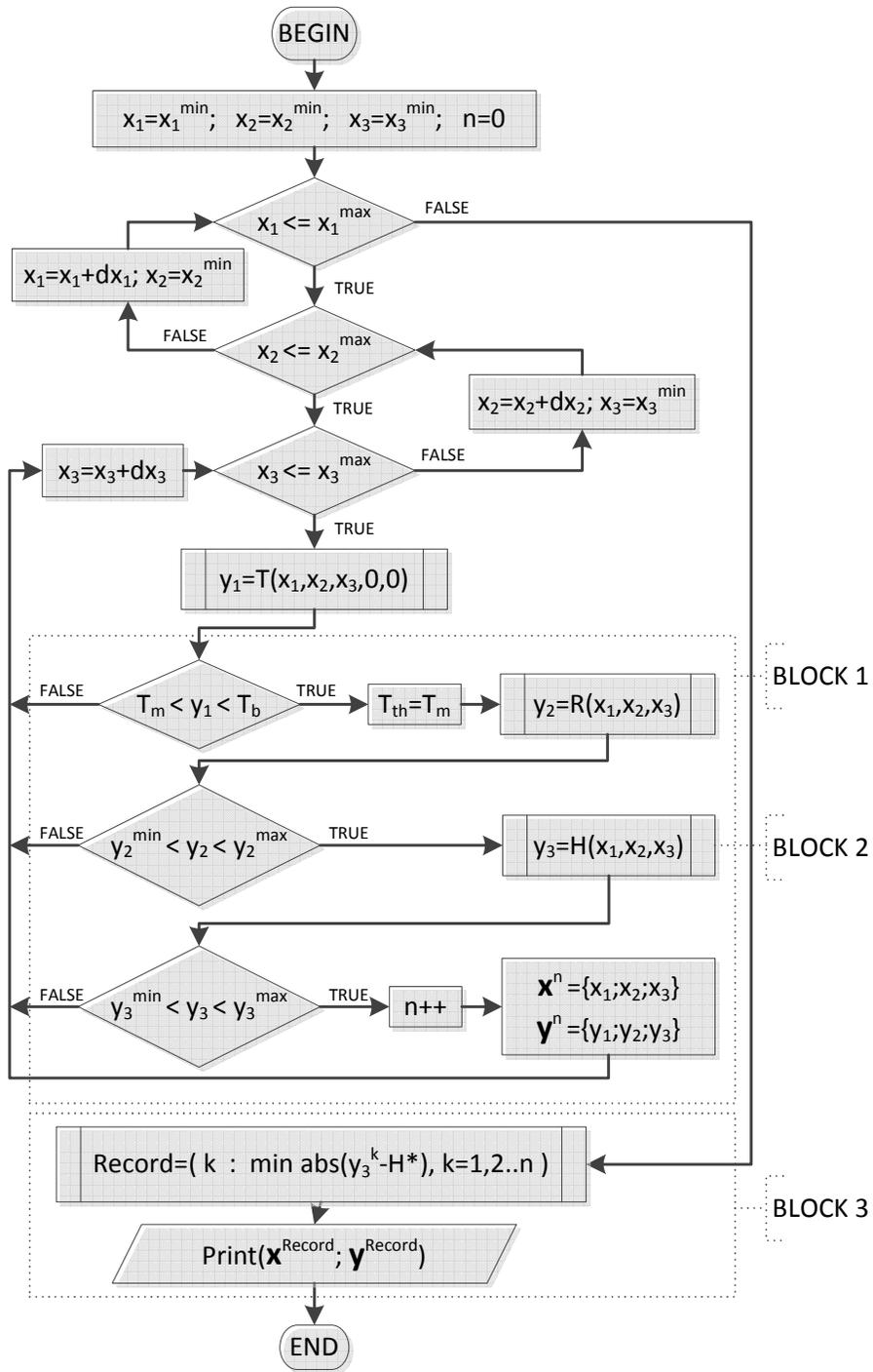
**Fig. 2.** The block diagram for solving of the problem about an optimal choice of variable parameters by scanning method of the search space
