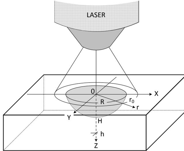
**Fig. 1.** Scheme of the molten pool obtained by thermal laser radiation:  $H$  – the depth of molten pool (melt depth);  $R$  – isotherm radius on the sample surface corresponding to the melting temperature  $T_m$ ;  $r_0$  – the radius of the laser spot on the sample surface;  $h$  – the sample thickness
