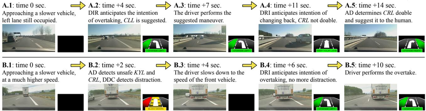
Figure 3: Two examples of the system on the prototype vehicle, showing the external camera view and the HMI.
