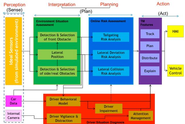
Figure 1: prototype architecture implemented in the demonstrator.
