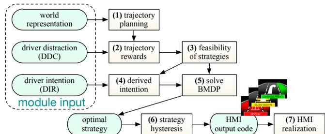
Figure 2: logic-flow of the co-pilot module for decision-making.
